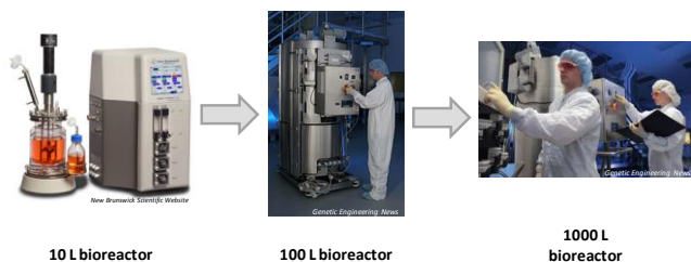
Figure 7. Diagram of a microcarrier-based scale up manufacturing
